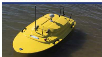
REMOTE HYDROGRAPHIC SURVEY BOAT
